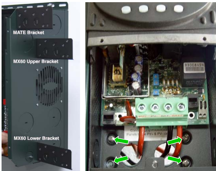
Figure 16. Brackets for MATE & MX60 (left) & lower 4 screw positions for MX60 (right).
