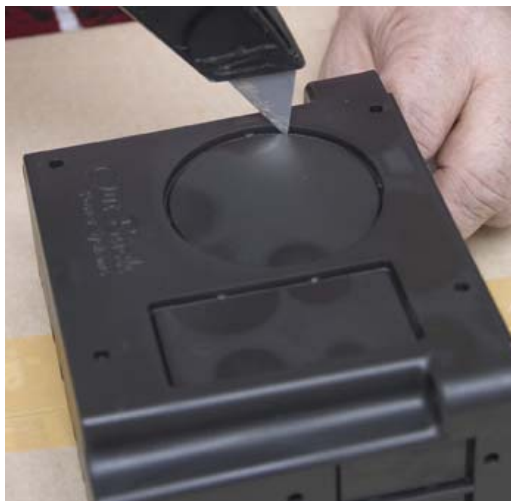
Figure 6. Cut the 2 1/2" circle out of the plastic FX-ACAS.
